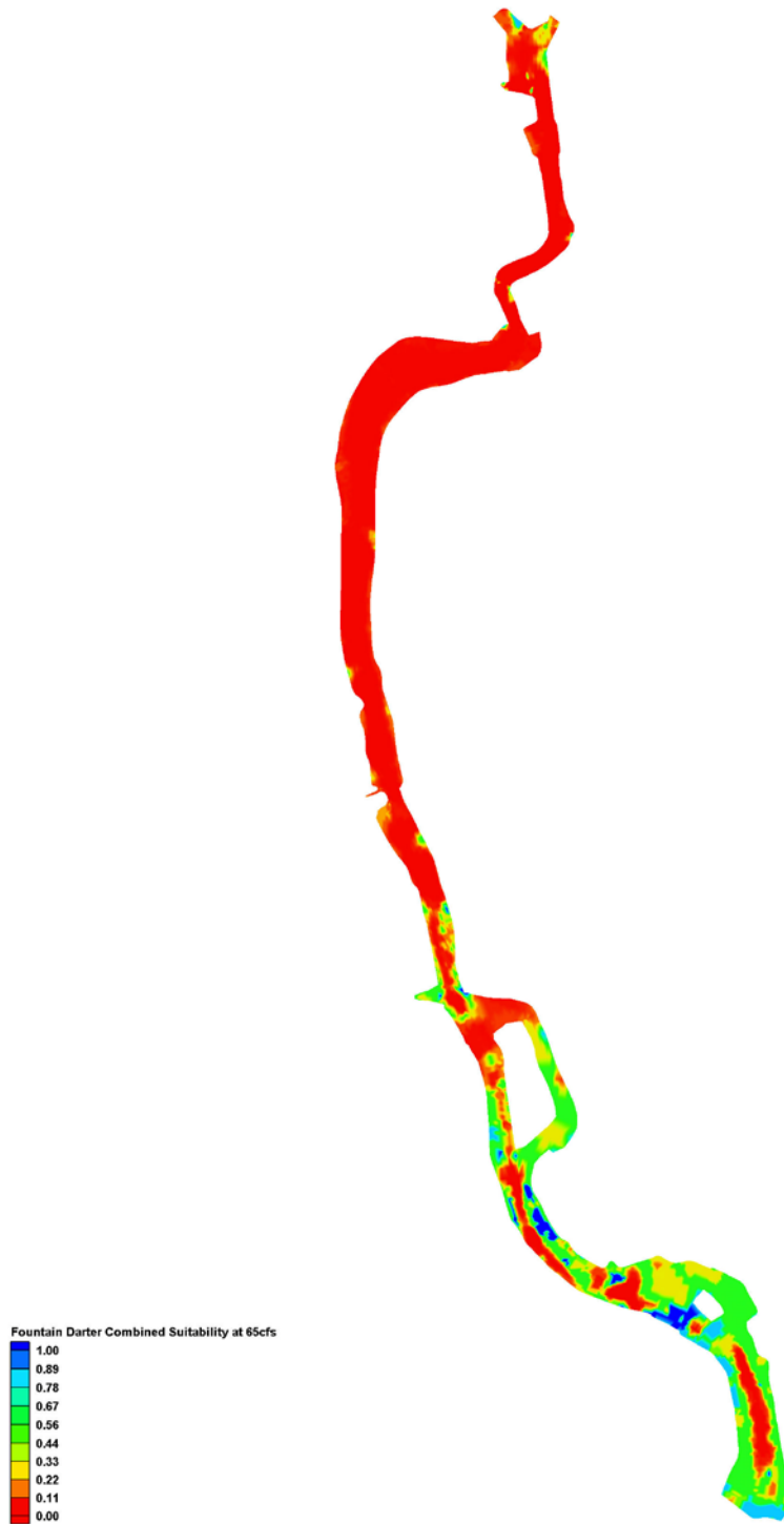
Figure 54. Combined suitability for fountain darter habitat in the Spring Lake to Rio Vista section of the San Marcos River at 65 cfs.
