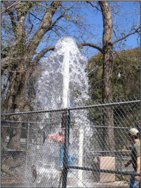
Figure 49. Artesian flow at the LCRA well.
