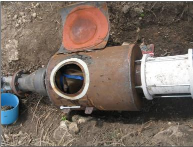
Figure 78. Inline barrel sampler in the irrigation line at the Tschirhart Well.
