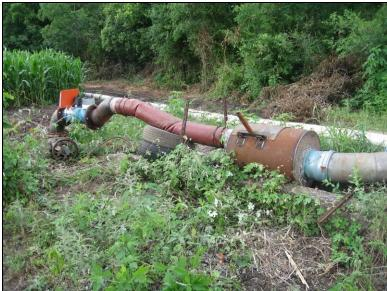
Figure 61. A barrel sampler was installed on the Persyn Well.
