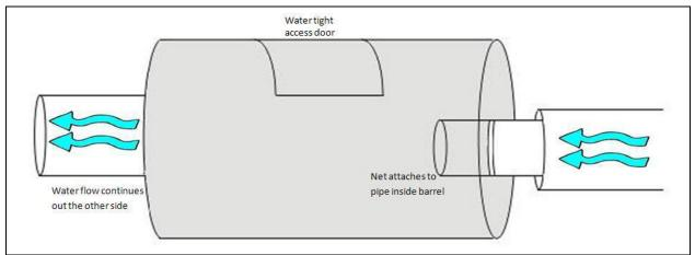
Figure 4. Schematic of in-line barrel sampler.
