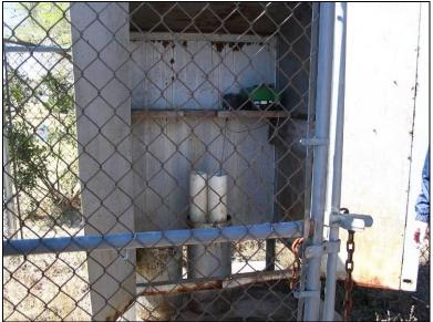
Figure 69. The San Marcos Flagpole Well was only large enough to drop a bottle trap into. There was no flow at this site.
