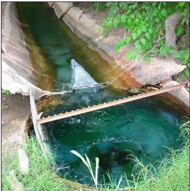
Figure 88. The Verstuyft Farms Well outlet is located at the bottom of this aqueduct head, and one method of sampling involved securing a net in the path of the water downstream of the outlet (shown).
