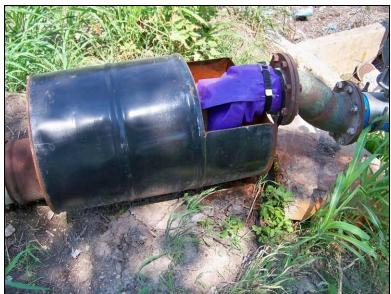
Figure 62. An open barrel style sampler was used to samplethe Raymond Wauters Well in 2009.
