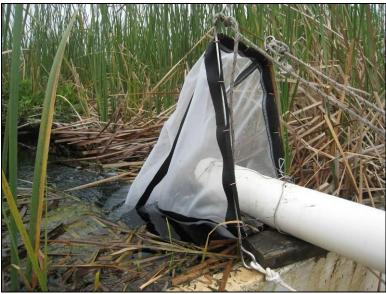
Figure 2. Framed net on nursery tank outflow at the Aldridge 209 Well.
